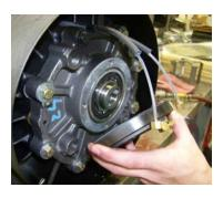
3. Remove the four (4) bolts that hold the rear bearing cover to the rear endplate and note that the wave spring seal is to be re-used.
