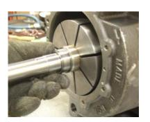
Use a welding glove to take the hot inner race from the hot plate and slide it onto the rotor shaft.
