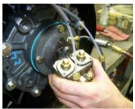
2. Remove the oil line guard. Disconnect all oil lines feeding from the oil pump
