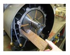
7. Remove the rear endplate, gasket, and vanes.
