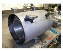
12. Remove the four-way assembly, gaskets, and check valve assembly. Carefully turn the housing upside down so that the pump feet are facing the ceiling.
