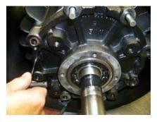
23. Insert one (1) of the dowel pin "T-handles" into either of the dowel pin holes on the endplate through into the housing.
