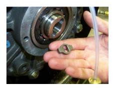
4. Remove the oil pump drive key from the end of the rotor.
