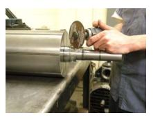
15. (Optional) If there is damage evident to the bearings, they will need to be replaced. Once the rotor is removed, start by cutting off the old bearing inner race on both ends of the rotor. Be sure to line up the cutting wheel with one of the vane slots so as not to damage the rotor or seal sleeve.
