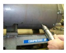
5. (Fan Cooled Only) Remove the eleven (11) self-tapping screws that fasten the fan shroud "tin" to the pump. Remove the fan shroud support connecting the fan shroud "tin" to the rear endplate.
