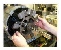
(Fan Cooled Only) Remove the fan guard on the drive end side of the pump. Remove the fan and key from the rotor drive end by first loosening the fan hub screw. You may find it necessary to drive the hub apart with a screw driver in order to slide the fan assembly off of the rotor.
