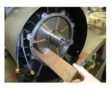
7. Remove the rear endplate with a gentle "wiggle", clean gasket surface and remove the vanes for inspection.
