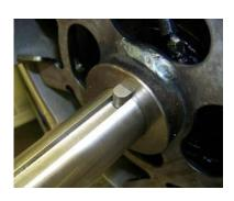
27. (Fan Cooled Only) Reinstall the fan assembly, the key should be pushed all the way to the end of the key slot on the drive end.
