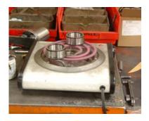
17. (Continuation of Step 15) Remove the two (2) inner races from the replacement bearings provided in your repair kit.
