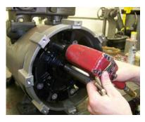
10. Repeat step 6 to drop the rear end of the rotor down onto the cushion.
