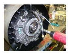
6. Remove the top two endplate bolts and replace with two (2) 3/8-16 stud/ dowels (or de-headed bolts), and then remove the remaining bolts.
