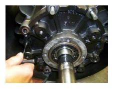
10. Insert the two (2) "T-handle" pins provided in your rebuild kit through the endplate and into the locator holes at 3 and 6 O'clock positions on the housing.
