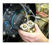
2. Remove the oil line guard. Disconnect all oil lines feeding from the oil pump
