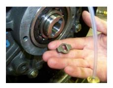
Remove the oil pump drive key from the end of the rotor.
