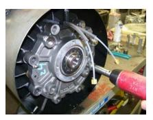
6. Remove the top two (2) bolts that hold the rear endplate to the pump housing and replace with two (2) 3/8-16 threaded dowels. Once in place, remove the lower six (6) 3/8 hex bolts.
