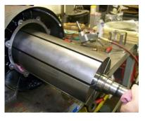
11. Gently guide the front endplate off of the (2) 3/8-16 threaded rod segments to fully settle the rotor body on the base of the housing bore.
