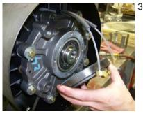
Remove the four (4) bolts that hold the rear bearing cover to the rear endplate and remove the rear bearing cover.
